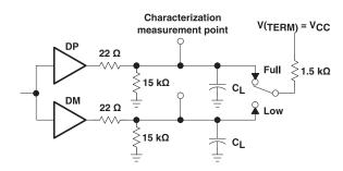
Figure 1. Differential Driver Switching Load
