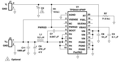
Figure 10. TPS54314 Schematic
