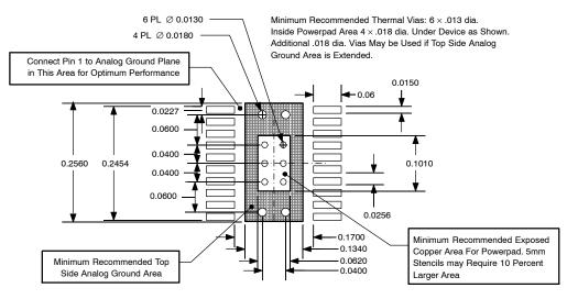
Figure 12. Recommended Land Pattern for 20-Pin PWP PowerPAD
