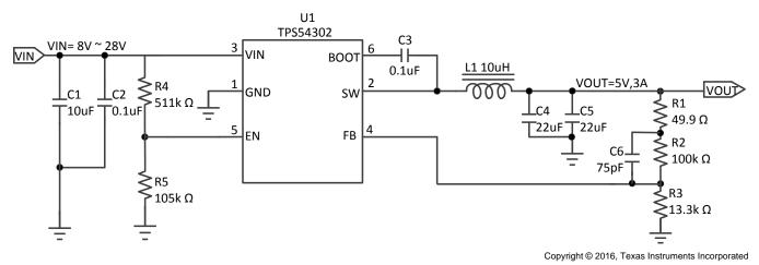
Figure 15. 5-V, 3-A Reference Design
