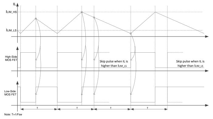
Figure 14. Overcurrent Protection for Both MOSFETs
