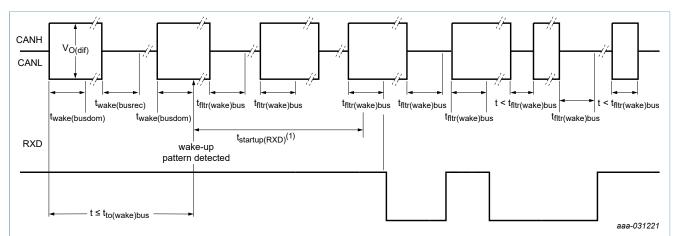
(1) During  $t_{startup(RXD)}$ , the low-power receiver is on but pin RXD is not active (i.e. HIGH/recessive). The first dominant pulse of width  $\geq t_{fltr(wake)bus}$  that ends after  $t_{startup(RXD)}$  will trigger RXD to go LOW/dominant.
