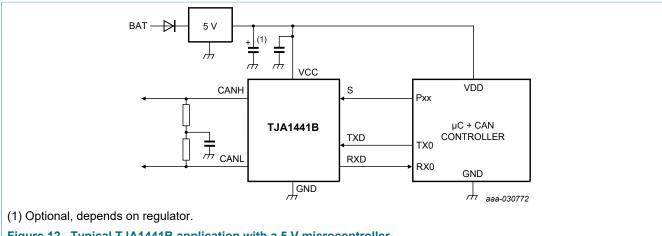
Figure 12. Typical TJA1441B application with a 5 V microcontroller
