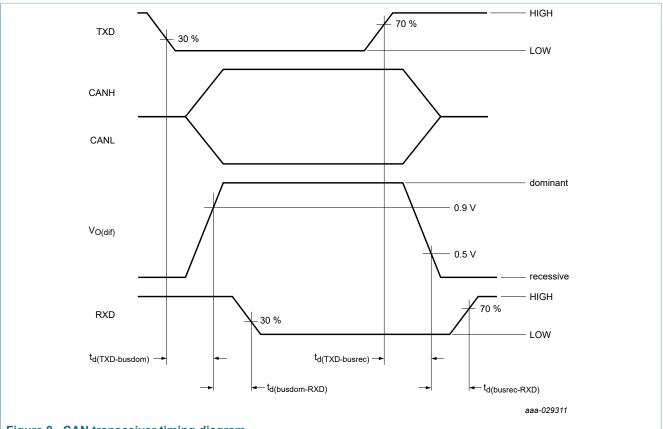
Figure 8. CAN transceiver timing diagram
