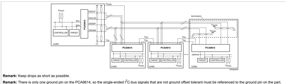
And any ground offset must be on the differential side where the differential input and output can tolerate a ground offset of up to 0.5 × V<sub>DD(B)</sub>.
