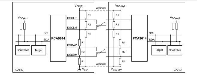
Figure 6. Typical application for PCA9614
