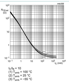
Fig. 13. Collector-emitter equivalent on-resistance as a function of collector current; typical values
