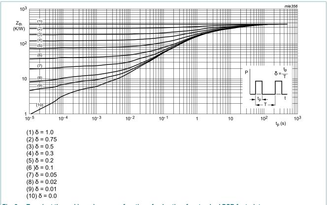
Fig. 2. Transient thermal impedance as a function of pulse time for standard PCB footprint
