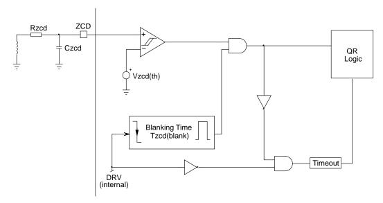
Figure 51. Valley Lockout Detection Circuitry Internal Schematic
