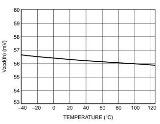
Figure 27. V<sub>ZCD(th)</sub> vs. Junction Temperature
