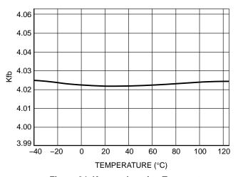
Figure 24. K<sub>FB</sub> vs. Junction Temperature
