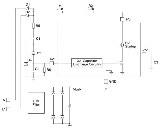
Figure 48. Simplified Block Diagram of X2 Capacitor Discharge Circuitry
