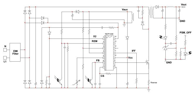
Figure 2. NCP1339 Typical Application Circuit (with IFF pin)
