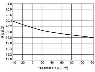
Figure 25. R<sub>FB</sub> vs. Junction Temperature
