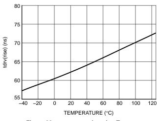
Figure 22. t<sub>DRV(rise)</sub> vs. Junction Temperature
