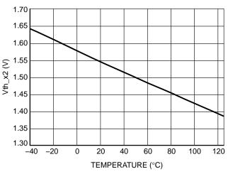
Figure 13. V<sub>th x2</sub> vs. Junction Temperature
