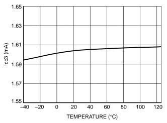
Figure 12. ICC3 vs. Junction Temperature
