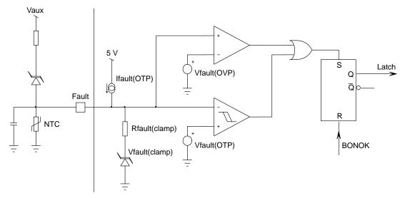
Figure 50. Fault Detection Schematic
