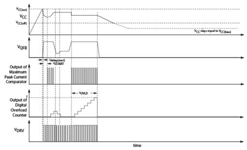
Figure 59. Latched Overload Operation
