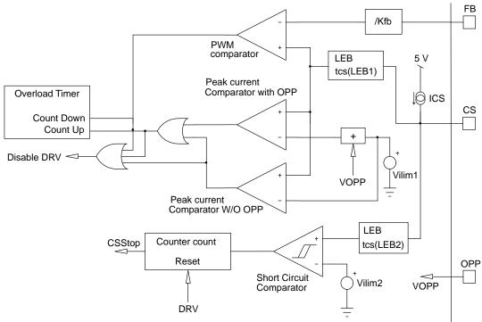
Figure 57. Overload Circuitry
