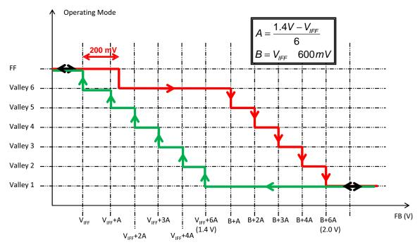
Figure 54. Valley Lockout Thresholds With IFF Pin
