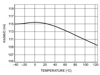
Figure 35. t<sub>CS(LEB2)</sub> vs. Junction Temperature
