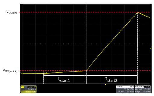
Figure 45. V<sub>cc</sub> at Start-up is made of Two Segments given the Short-circuit Protection Implemented on the HV Source
