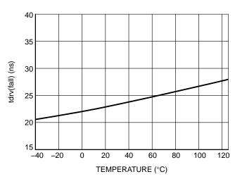
Figure 23. t<sub>DRV(fall)</sub> vs. Junction Temperature
