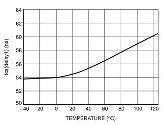
Figure 32. t<sub>CS(LEB1)</sub> vs. Junction Temperature
