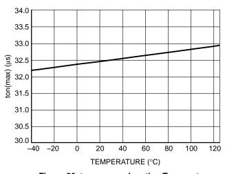
Figure 26.  $t_{on(MAX)}$  vs. Junction Temperature
