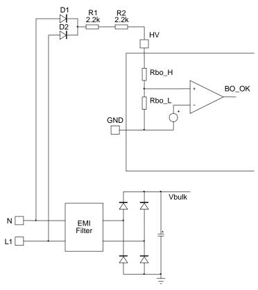
Figure 46. Simplified View of the Brown-out Circuitry
