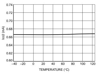
Figure 11. ICC2 vs. Junction Temperature
