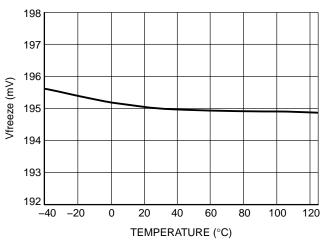
Figure 37. V<sub>freeze</sub> vs. Junction Temperature
