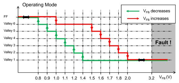
Figure 53. Valley Lockout Thresholds Without IFF Pin
