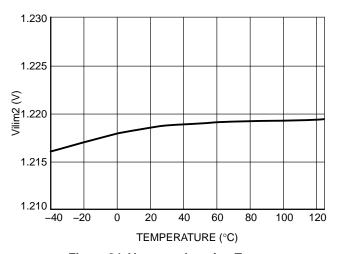
Figure 34. V<sub>ilim2</sub> vs. Junction Temperature
