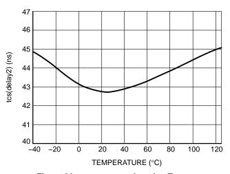
Figure 36. t<sub>CS(delav2)</sub> vs. Junction Temperature
