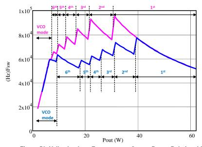
Figure 52. Valley Lockout Frequency vs Output Power Relationship
