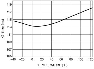
Figure 14. X2\_timer vs. Junction Temperature
