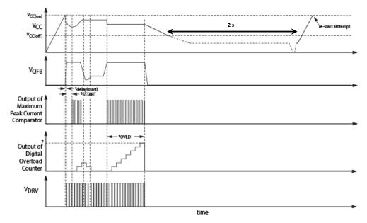
Figure 58. Auto-recovery Overload Operation
