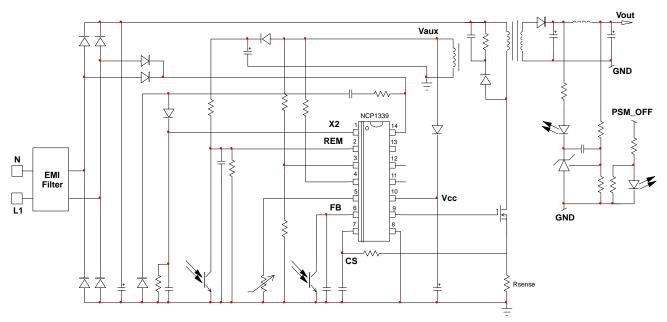
Figure 1. NCP1339 Typical Application Circuit (without IFF pin)
