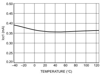
Figure 10. ICC1 vs. Junction Temperature
