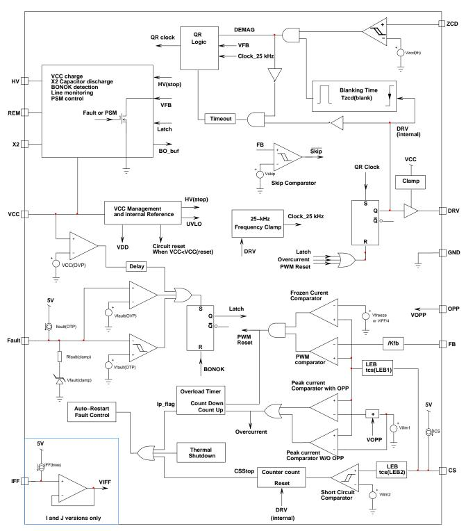
Figure 3. NCP1339 Functional Block Diagram
