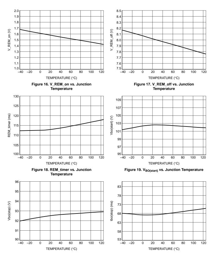
Figure 20. V<sub>BO(stop)</sub> vs. Junction Temperature
