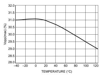
Figure 39. V<sub>OPP(MAX)</sub> vs. Junction Temperature
