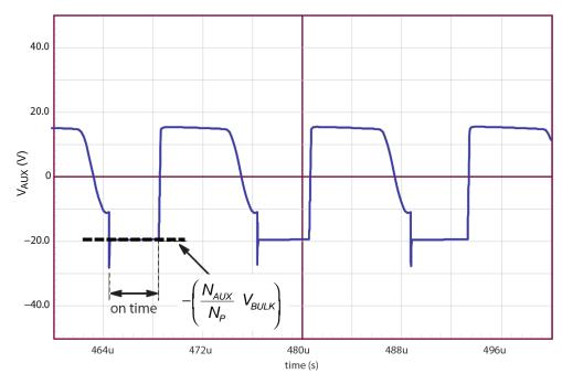
Figure 55. Auxiliary Winding Voltage Waveform
