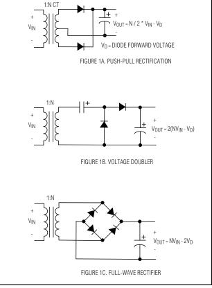
Figure 1. Secondary-Side Rectification Topologies
