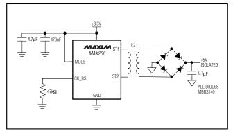
Figure 8b. +3.3V to Isolated +5V
