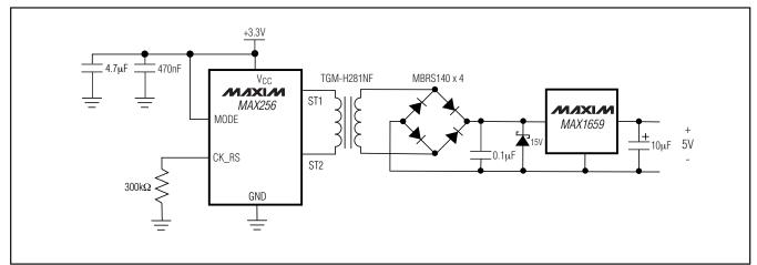
Figure 2. +3.3V to Isolated Regulated +5V
