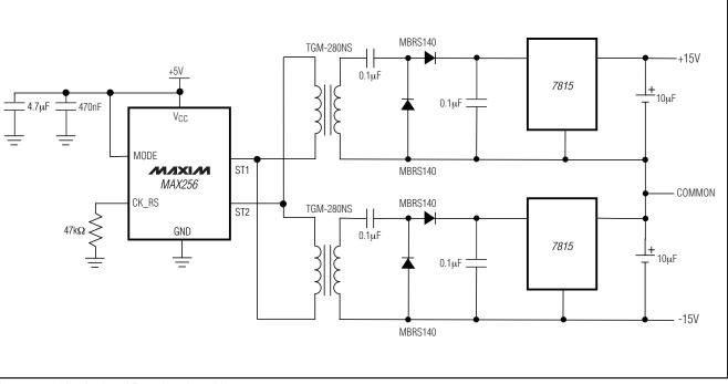
Figure 5. +5V to Isolated Regulated ±15V
