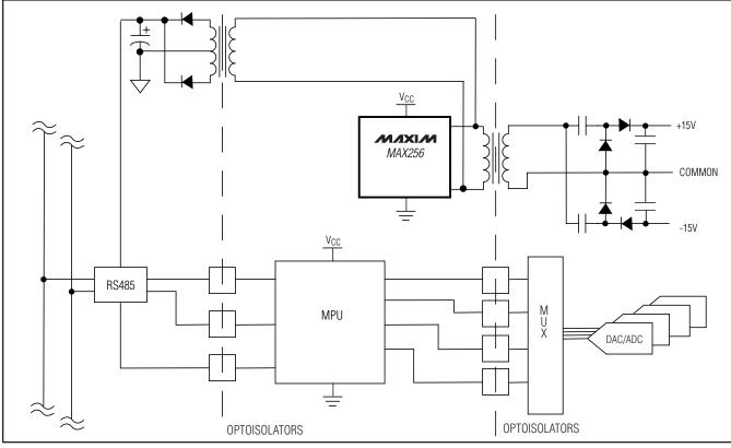
Figure 6. Isolated Power Supply for Process Control Applications
