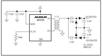
Figure 8c. +5V to Isolated ±15V
