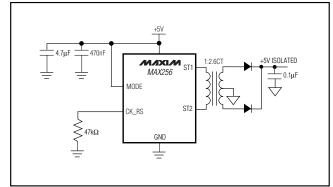
Figure 8a. +5V to Isolated +5V
