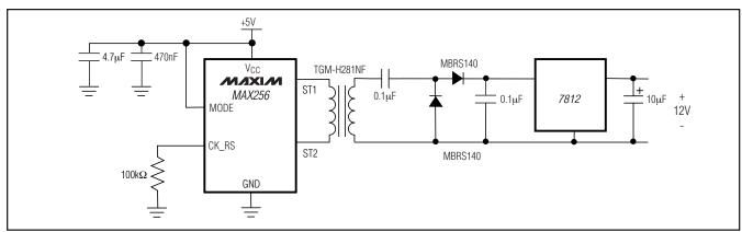
Figure 4. +5V to Isolated Regulated +12V
