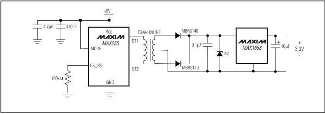
Figure 3. +5V to Isolated Regulated +3.3V
