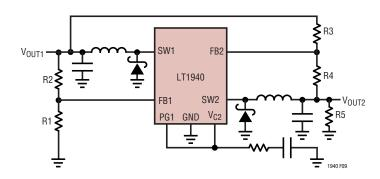
Figure 9. This circuit can be used when  $V_{OUT1}$  is greater than 1.25V and  $V_{OUT2}$  is less than 1.25V.
