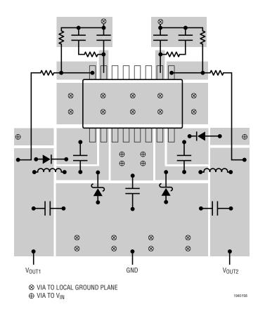
Figure 8. A Good PCB Layout Ensures Proper Low EMI Operation
