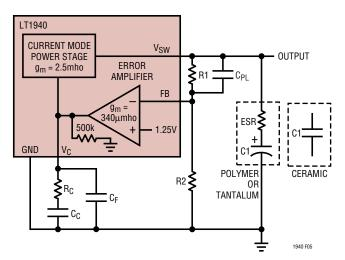
Figure 4. Model for Loop Response
