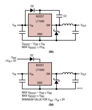
Figure 3. Generating the Boost Voltage
