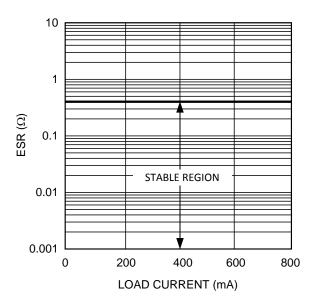
Figure 28. Stable Region for Output Capacitor ESR
