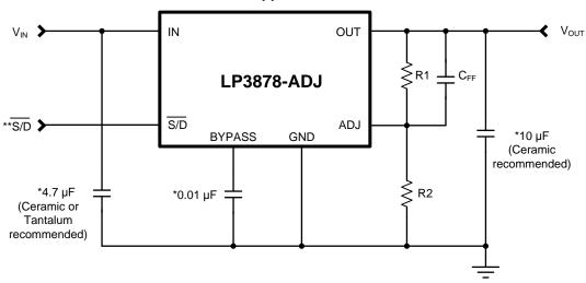
\*Capacitor values shown are minimum required to assure stability. A larger output capacitor provides improved dynamic response. Output capacitor must meet ESR requirements (see *Application Information*).
