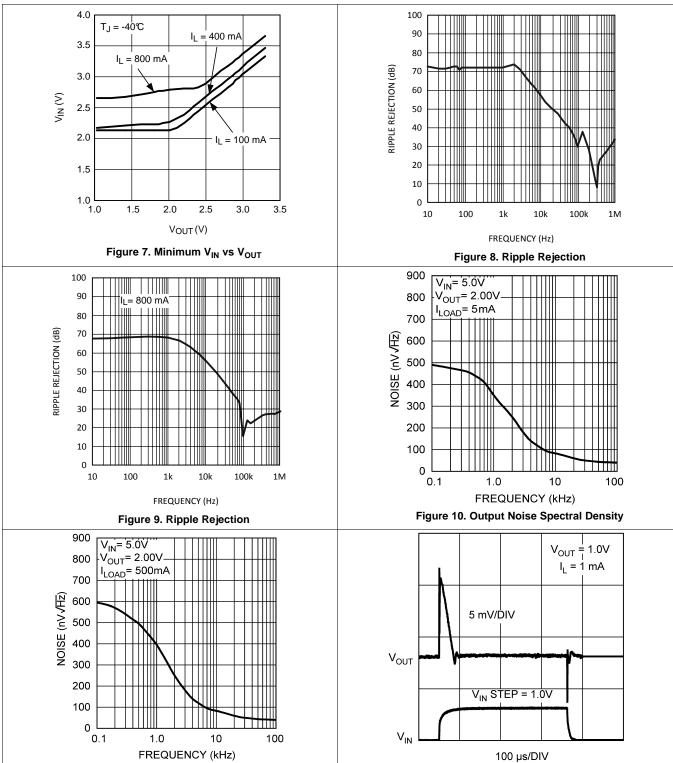
Figure 11. Output Noise Spectral Density
