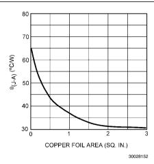
FIGURE 12.  $\theta_{\text{JA}}$  vs Copper Area for TO-263 Package
