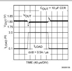
FIGURE 4. Load Transient Response: 10 µF Ceramic, 0.5A/µs di/dt
