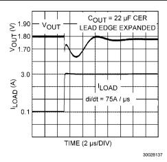
FIGURE 7. 22 µF Ceramic Output Capacitor
