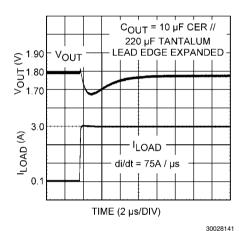
FIGURE 10. 10 uF Ceramic Paralleled By 220 uF Tantalum
