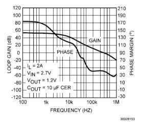
FIGURE 2. Gain-Bandwidth Plot for 2A Load
