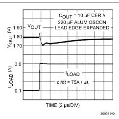
FIGURE 11. 10 µF Ceramic Paralleled By 220 µF OSCON
