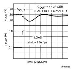
FIGURE 8. 47 µF Ceramic Output Capacitor
