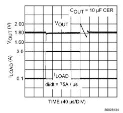
FIGURE 5. Load Transient Response: 10 µF Ceramic, 75A/µs di/dt
