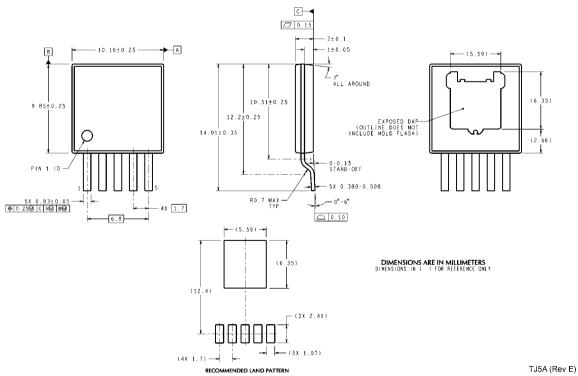
TO-263 THIN 5-Lead, Molded, Surface Mount Package NS Package Number TJ5A
