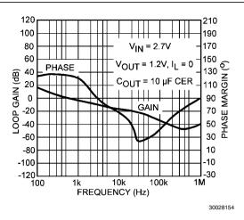
FIGURE 3. Gain-Bandwidth Plot for No Load
