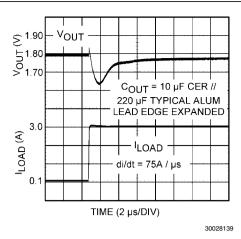
FIGURE 9. 10 µF Ceramic Paralleled By 220 µF Generic Aluminum Electrolytic
