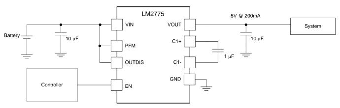
Figure 19. Typical LM2775 Configuration
