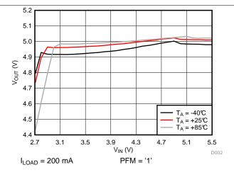
Figure 1. PWM Output Regulation
