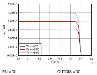
Figure 24. Output Leakage Current High Z
