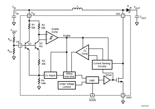
FIGURE 2. LM2704 Block Diagram
