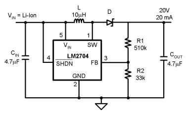
C<sub>IN</sub>: Taiyo Yuden Ceramic C<sub>OUT</sub>: Taiyo Yuden Ceramic L: Coilcraft DO1608C-103 D: Motorola MBRM130LT3
