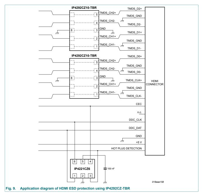
The device uses an advanced clamping structure showing a negative dynamic resistance. This snap-back behavior strongly reduces the clamping voltage to the system behind the ESD protection during an ESD event. Do not connect unlimited DC current sources to the data lines to avoid keeping the ESD protection device in snap-back state after exceeding breakdown voltage (due to an ESD pulse for instance).
