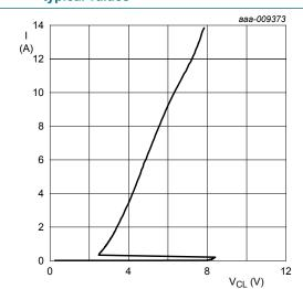
Dynamic resistance with positive clamping; Fig. 7. typical values
