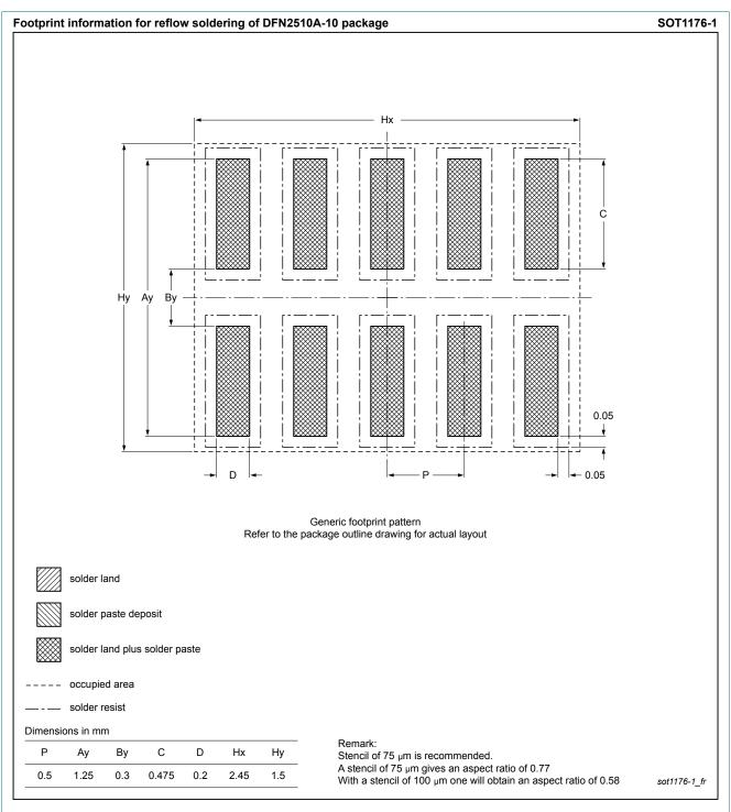
Fig. 11. Reflow soldering footprint for DFN2510A-10 (SOT1176-1)
