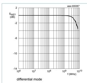
Fig. 1. Insertion loss; typical values
