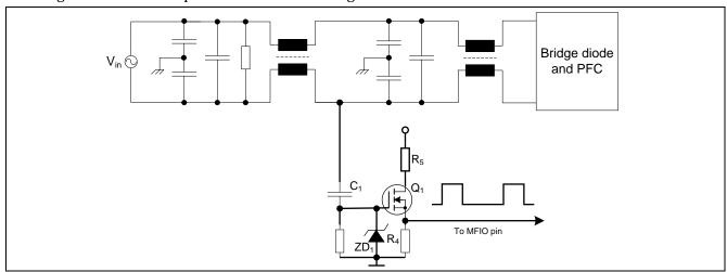
Circuit with AC detection with EMI filter Figure 9
