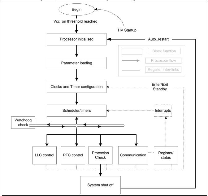
Figure 5 Overview of Processor operations
