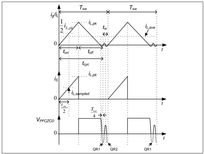
Figure 11 Current and timing in QR2 Operation
