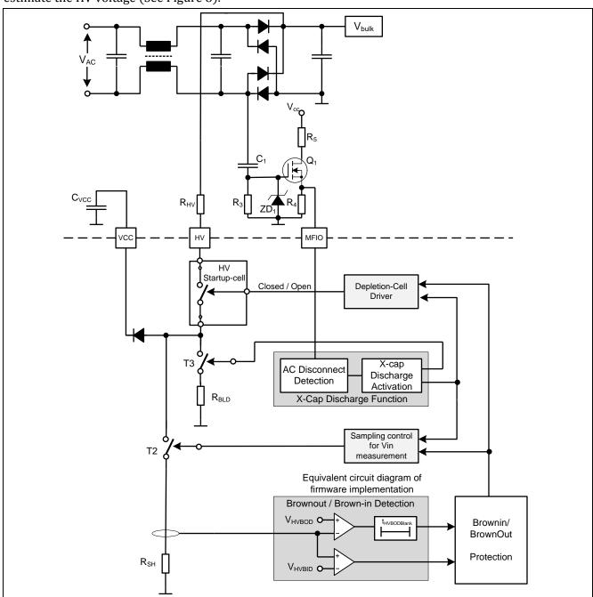
Figure 8 High voltage sensing at MFIO pin
