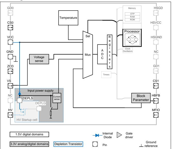
Voltage and current sensing multiplexing to ADC Figure 6
