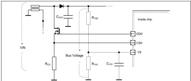
PFC control at GD0 pin and Voltage and current sensing at VS and CS pins Figure 10
