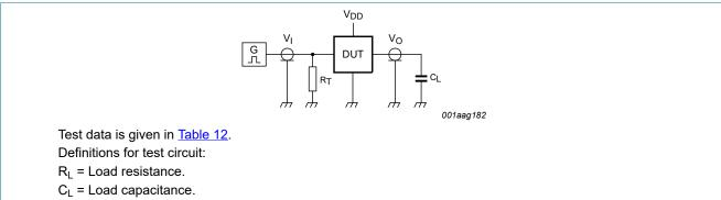
$R_T$  = Termination resistance should be equal to output impedance of  $Z_0$  of the pulse generator.
