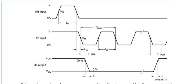
a. Pulse widths, maximum frequency, recovery and transition times, and A2 to Qn propagation delays
