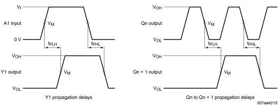
b. A1 to Y1, MR to Qn, and Qn to Qn + 1 propagation delays
