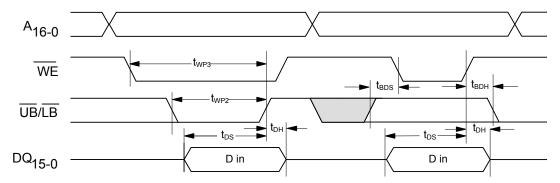
Figure 15. Page Mode Write Cycle Timing
