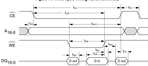
Figure 11. Write Cycle Timing 1 (WE Controlled) [9]
