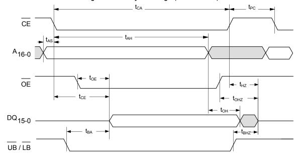
Figure 10. Page Mode Read Cycle Timing [8]
