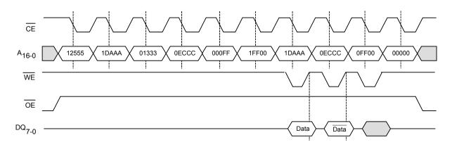
Figure 5. Sequence to Read Write-Protect Settings [1]
