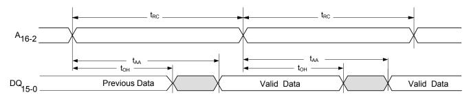
Figure 9. Read Cycle Timing 2 (CE Controlled)
