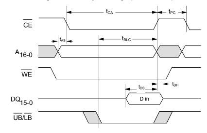
Figure 13. Write Cycle Timing 3 ( $\overline{\text{CE}}$  LOW) [9]
