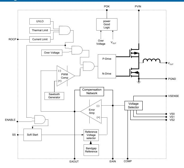
Figure 3. System block diagram.
