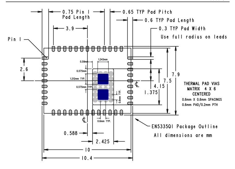
Figure 6: EN5335QI PCB Footprint (Top View)
