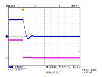
Start-up waveform,  $V_{IN}/V_{OUT} = 5.5V/1.2V$
