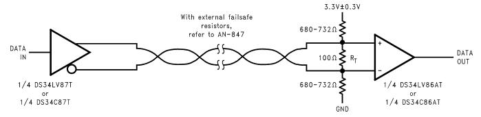
Figure 7. Typical Driver Connection
