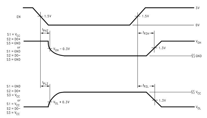
Figure 6. Driver Single-Ended Tri-state Waveforms
