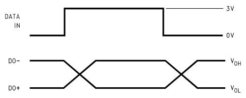
Figure 8. Typical Driver Output Waveforms
