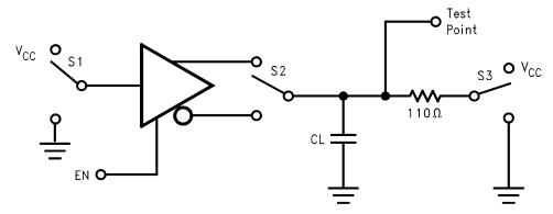
Figure 5. Driver Single-Ended Tri-state Test Circuit
