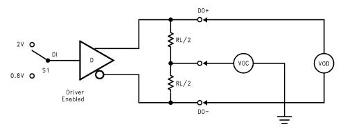
Figure 2. Differential Driver DC Test Circuit
