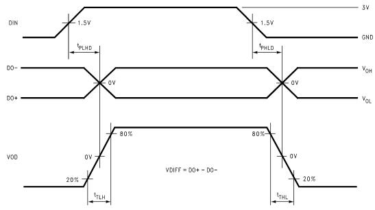
Generator waveform for all tests unless otherwise specified: f = 1 MHz, Duty Cycle = 50%,  $Z_0 = 50\Omega$ ,  $t_f \le 10$  ns,  $t_f \le 10$  ns.
