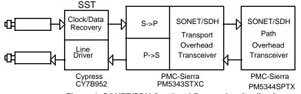
Figure 1. SONET/SDH Overhead Processing Application
