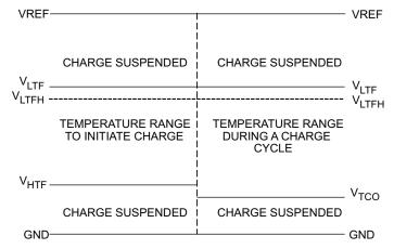
Figure 17. TS pin, Thermistor Sense Thresholds
