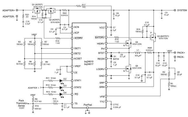
VIN=19V, 3-cell, I<sub>adapter limit</sub>=4A, I<sub>charge</sub>=3A, I<sub>pre-charge</sub>= I<sub>term</sub>=0.3A, 5 hour saftey timer
