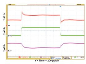
Figure 9. Transient System Load (DPM)
