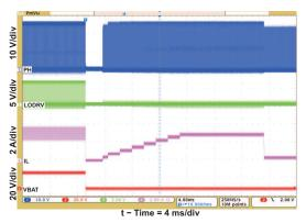
Figure 11. Battery to GND Short Protection
