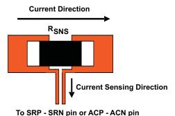
Figure 23. Sensing Resistor PCB Layout
