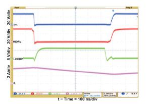
Figure 6. Continuous Conduction Mode Switching Waveform
