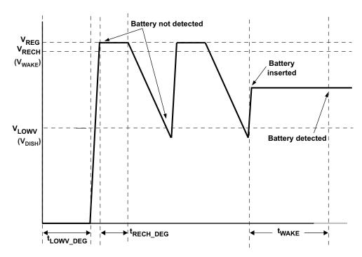
Figure 20. Battery Detect Timing Diagram
