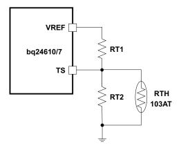
Figure 18. TS Resistor Network
