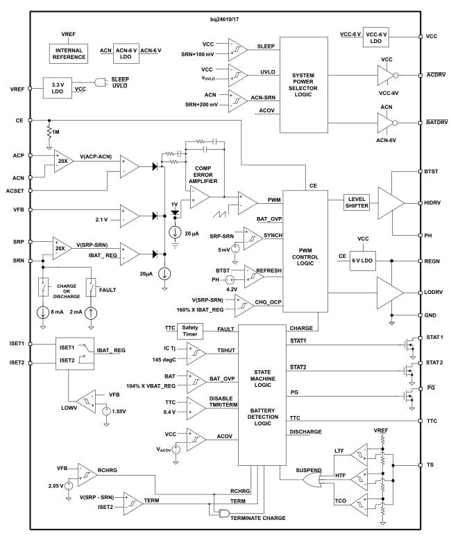
Figure 14. Functional Block Diagram for bq24610/7
