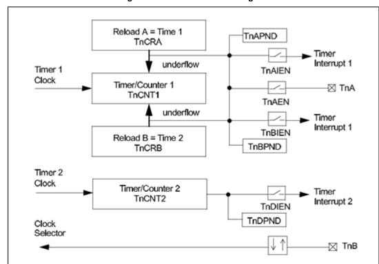
Figure 12: MFT mode 1 block diagram
