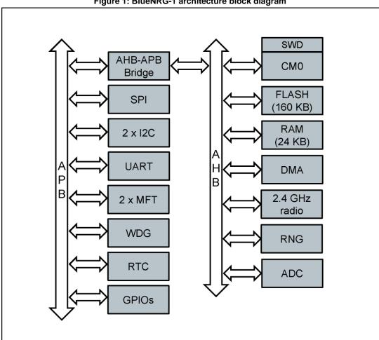
Figure 1: BlueNRG-1 architecture block diagram
