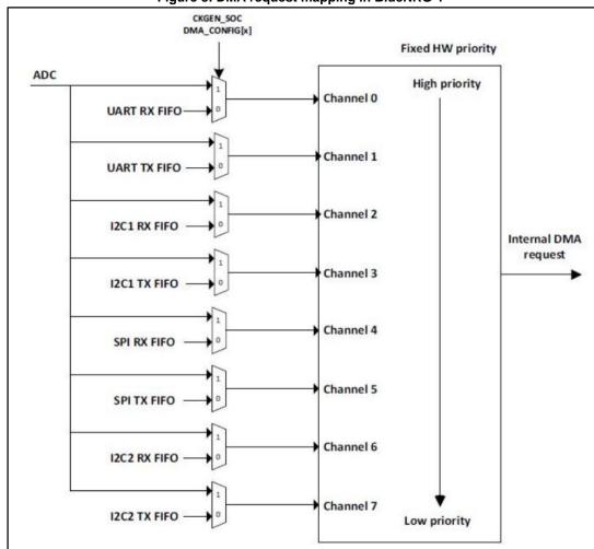
Figure 8: DMA request mapping in BlueNRG-1
