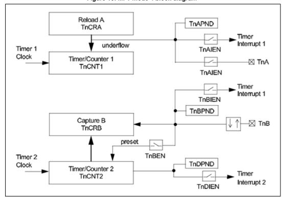
Figure 16: MFT mode 4 block diagram
