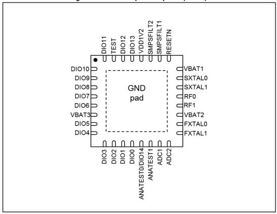
Figure 17: BlueNRG-1 pin out top view (QFN32)
