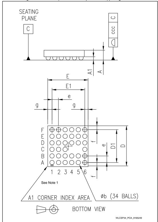
The corner of terminal A1 must be identified on the top surface by using a laser marking dot.
