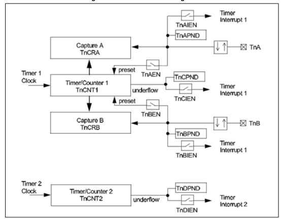
Figure 14: MFT mode 2 block diagram
