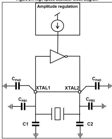
Figure 24: High speed oscillator block diagram
