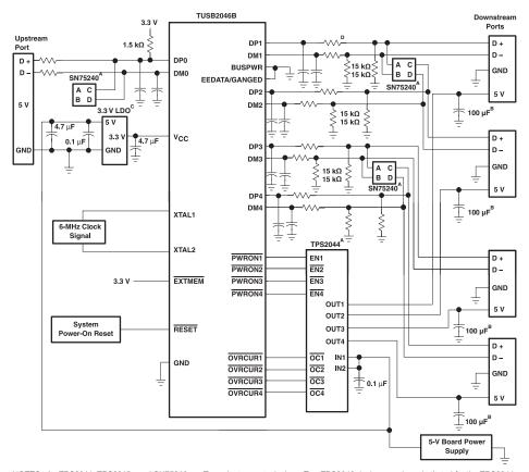
NOTES: A. TPS2044, TPS2042, and SN75240 are Texas Instruments devices. Two TPS2042 devices can be substituted for the TPS2044. The OCn outputs of the TPS204n are open drain. A 10-kΩ pullup is recommended.
