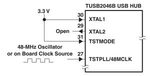
Figure 7. 48-MHz Input Clock Configuration
