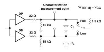
Figure 1. Differential Driver Switching Load
