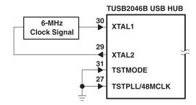
Figure 5. 6-MHz Input Clock Configuration
