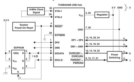
Figure 8. Typical Application of the TUSB2046x USB Hub
