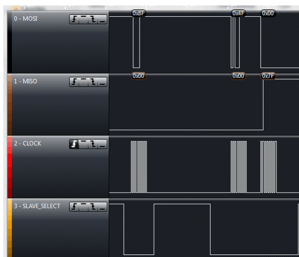
Figure 6-26. Reset FIFO and Read RSSI
