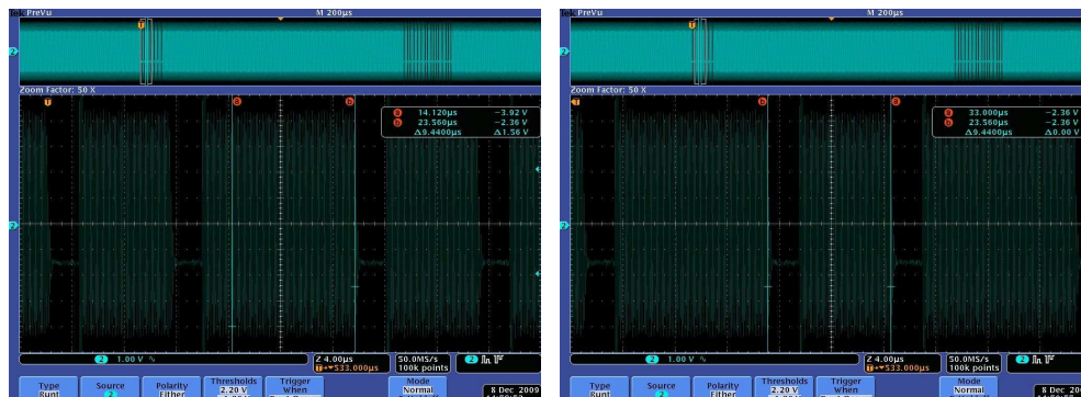
Figure 6-31. Receive Data Bits and Framing Level
