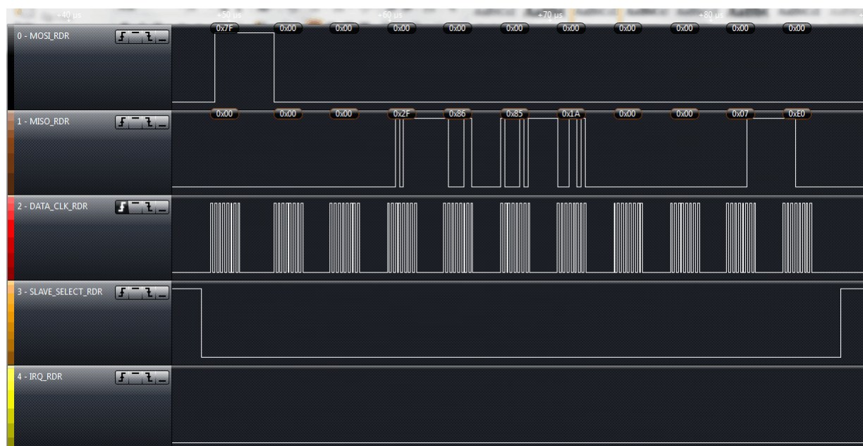
Figure 6-25. Continuous Read of FIFO After Inventory Command
