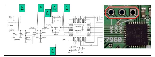
9. If the system implementation is complex (for example, if the RFID reader module is a subsystem of a larger system with other modules such as *Bluetooth*<sup>®</sup>, Wi-Fi<sup>®</sup>, microprocessors, and clocks), special considerations should be taken to ensure that no noise is coupled into the supply lines.
