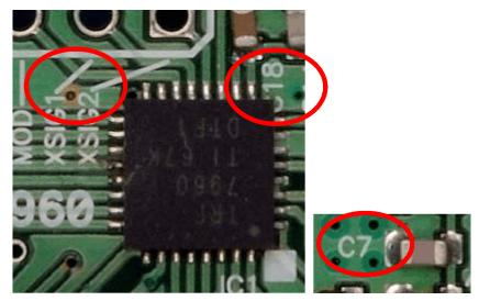
3. Place the two inductors at 90° orientations with respect to each other (that is, if the first inductor is laid out in a horizontal orientation, the next inductor should be placed in a vertical orientation). This arrangement minimizes coupling between the two inductors.
