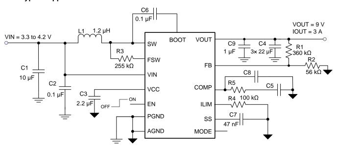
Figure 11. TPS61088 3.3 V to 9-V/3-A Output Converter
