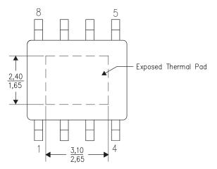
Figure 15. Thermal Pad Dimensions (Top View)
