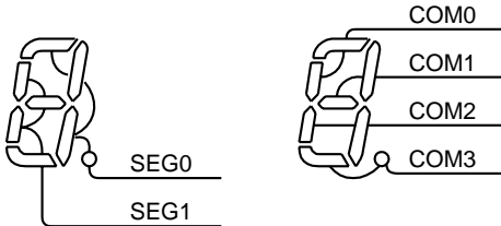
Figure 15-6 Example of COM, SEG Pin Connection (1/4 Duty)
