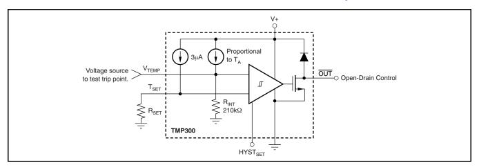
Figure 8. Applying Voltage to Trip Digital Output
