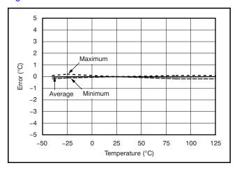
Figure 12. 5°C Hysteresis Error vs Temperature
