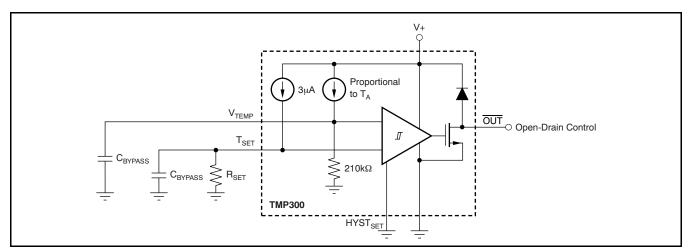
Figure 14. Bypass Capacitors Prevent Early Comparator Toggling Due to Circuit Board Noise
