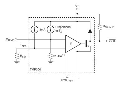
NOTE: (1) Thinfilm resistor with approximately 10% accuracy; however, this accuracy error is trimmed out at the factory.
