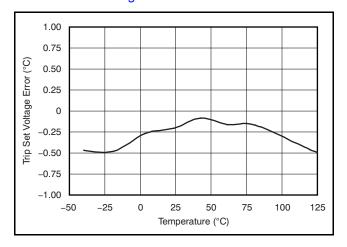
Figure 10. Trip Set Voltage Error vs Temperature
