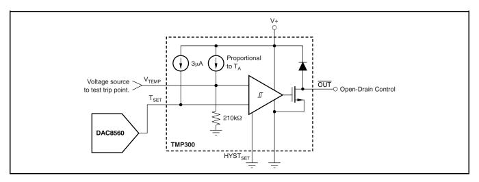
Figure 11. DAC Generates the Voltage-Driving T<sub>SET</sub> Pin
