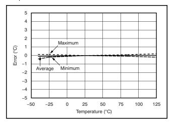
Figure 13. 10°C Hysteresis Error vs Temperature
