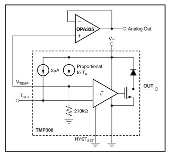
Figure 9. Buffering the Analog Output Signal
