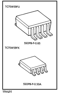
Weight SSOP8-P-0.65: 0.021g (typ.) SSOP8-P-0.50A: 0.01g (typ.)
