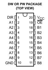
This device allows data transmission from the A bus to the B bus or from the B bus to the A bus, depending on the logic level at the direction-control (DIR) input. The output-enable  $(\overline{OE})$  input can be used to disable the device so that the buses are effectively isolated.
