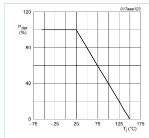
Fig. 2. Normalized total power dissipation as a function of junction temperature
