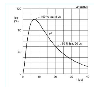
8/20 µs pulse waveform according to Fig. 2. IEC 61000-4-5
