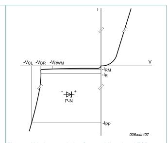
Fig. 5. V-I characteristics for a unidirectional ESD protection diode
