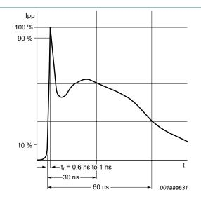
Fig. 3. ESD pulse waveform according to IEC 61000-4-2
