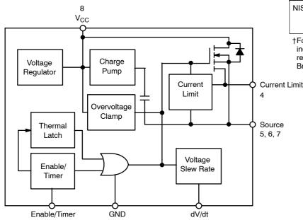
Figure 1. Block Diagram
