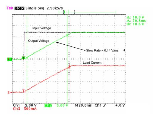
Figure 5. Turn–on Waveforms for a Resistive Load of 10  $\Omega$  (C<sub>dV</sub>/<sub>dt</sub> = 1  $\mu f)$
