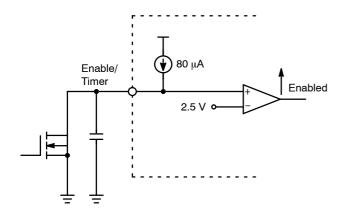
Figure 10. Simplified Schematic Diagram of the Enable/Timer Circuit
