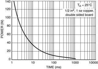
Figure 3. Overload vs. Shutdown Time
