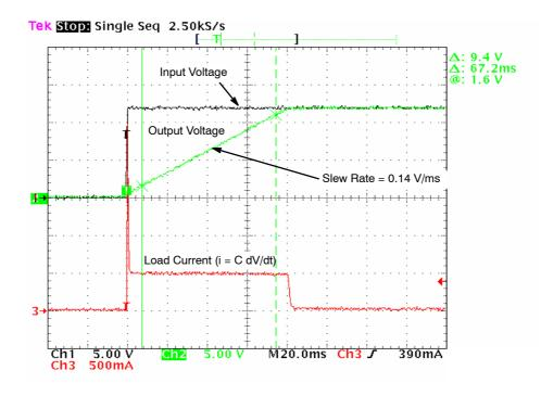
Figure 6. Turn-on Waveforms for a Load Capacitance of 3,300  $\mu f$  (C<sub>dV</sub>/<sub>dt</sub> = 1  $\mu f$ )
