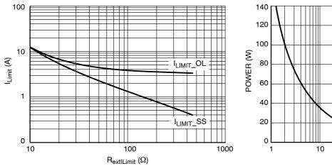
Figure 2. Current Limit Adjustment
