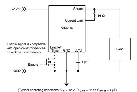
Figure 4. Typical Application Circuit
