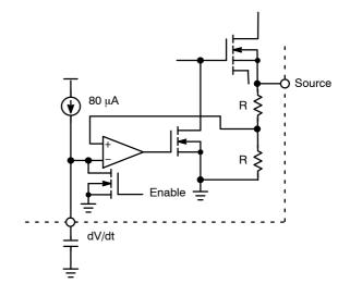
Figure 9. dV/dt Circuit
