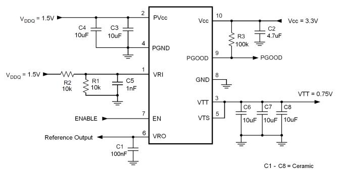
Figure 1. Typical DDR-3 Application Schematic
