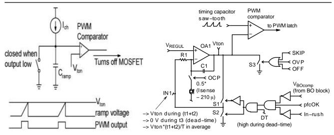
Figure 6. PWM Circuit and Timing Diagram
