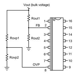
Figure 15. Configuration with Two Separate Feed-back Networks
