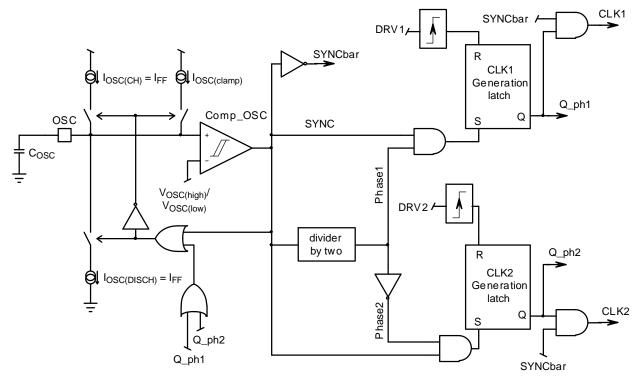
Figure 16. Oscillator Block
