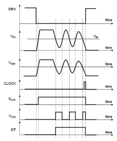
Figure 12. Zero Current Detection Timing Diagram (V<sub>AUX</sub> is the Voltage Provided by the ZCD Winding)
