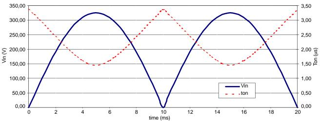
Figure 8. Input Voltage and On-time vs. Time (example with F<sub>SW</sub> = 100 kHz, Pin = 150 W, V<sub>AC</sub> = 230 V, L = 200 μH)
