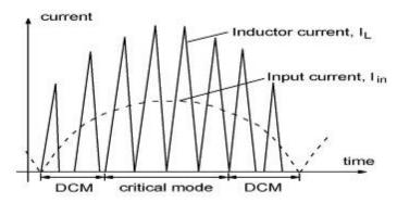
Figure 3. DCM and CRM Operation Within a Sinusoid Cycle for One Branch
