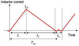
Figure 5. Inductor Current in DCM
