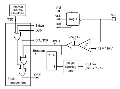
Figure 20. Fault Management Block
