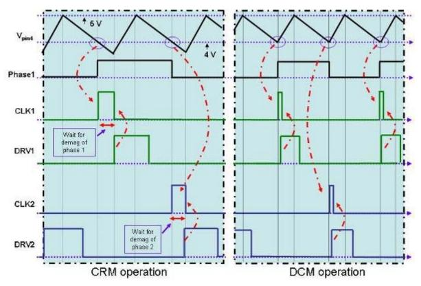
Figure 17. Typical Waveforms (T<sub>delay</sub> not shown here for the sake of simplicity)
