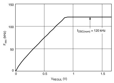
Figure 18. Fold-back Characteristic of the Clamp Frequency with  $R_{FF}$  = 8.2 k $\Omega$  and  $f_{OSC(nom)}$  = 120 kHz
