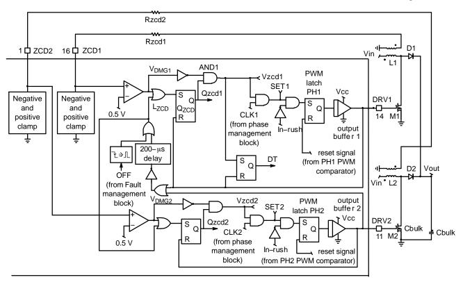
Figure 11. Zero Current Detection
