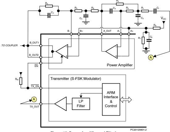
Figure 17. Power Amplifier and Filtering
