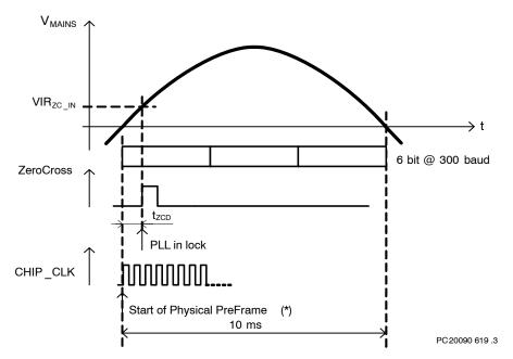
\*The start of the Physical Subframe is shifted back with  $R_ZC_ADJUST$ [7:0] x 13  $\mu$ S =  $t_{ZCD}$  to compensate for the zero cross delay.
