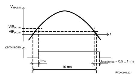
Figure 11. Zero Cross Detector Signals and Timing (example for 50 Hz)
