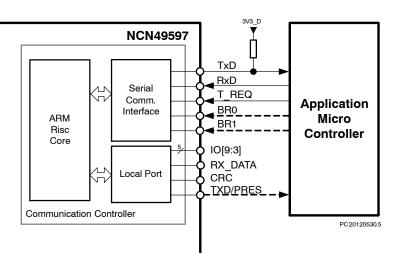
Figure 27. Connection to the Application Microcontroller
