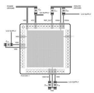
Figure 3: Recommended Layout of the Placement of Decoupling Capacitors
