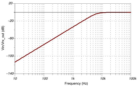
Figure 23. Transfer Function of 50 Hz Suppression Circuit
