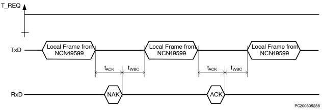
Figure 30. Transfer from NCN49599 to Application Micro Controller
