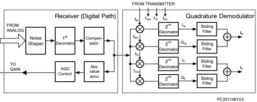
Figure 21. Digital Path of the Receiver ADC and Quadrature Demodulation
