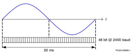
Figure 8. Data Stream is in Sync with Zero Cross of the Mains (example for 50 Hz)
