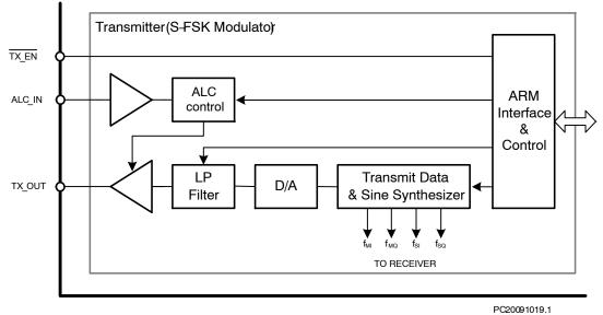
Figure 15. Transmitter Block Diagram
