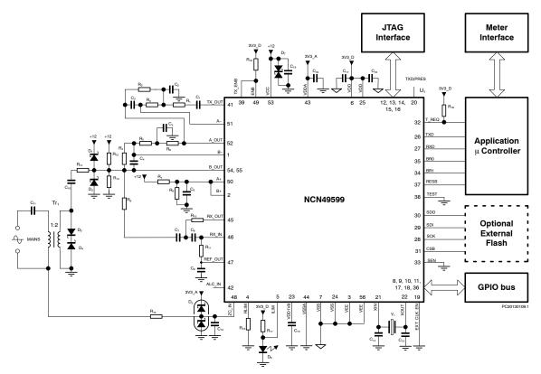
Figure 1. Typical Application for the NCN49599S-FSK Modem
