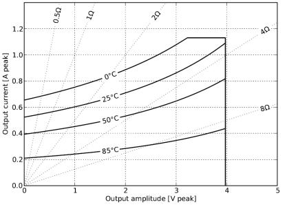
Figure 18. SOA in V<sub>L</sub>–IL space (bottom left corner is safe) with  $R_{thJA}$  = 50 K/W
