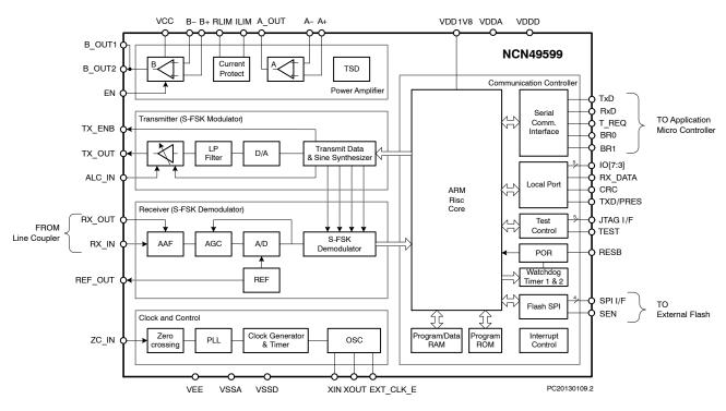
Figure 7. S-FSK Modem NCN49599 Block Diagram
