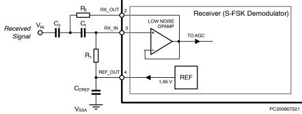
Figure 22. External Component Connection for 50/60 Hz Suppression Filter
