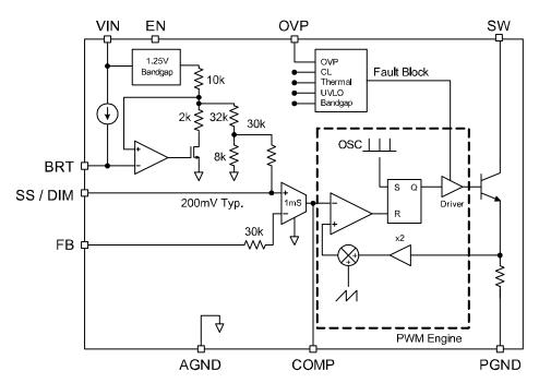
Figure 2. MIC2298 Block Diagram
