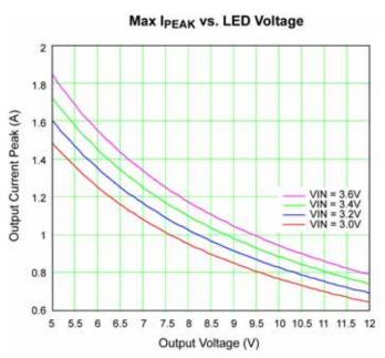
Figure 8. Peak Output Current vs.  $V_{\text{OUT}}$
