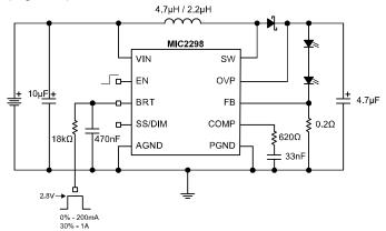
Figure 5. High Frequency PWM Programming
