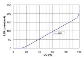
Figure 6. LED Current vs. DC (on enable pin)
