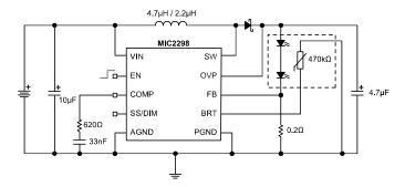
Figure 10. LED Thermal Protection
