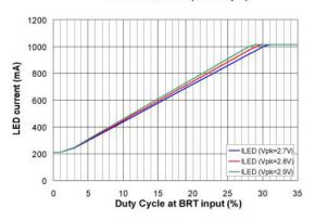
Figure 7. LED Current vs. DC (on BRT pin)
