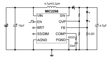
Figure 4. Adjustable OVP Circuit
