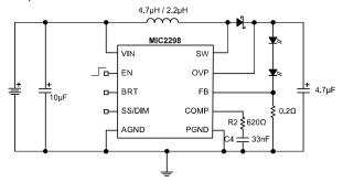
Figure 3. Typical Application Circuit
