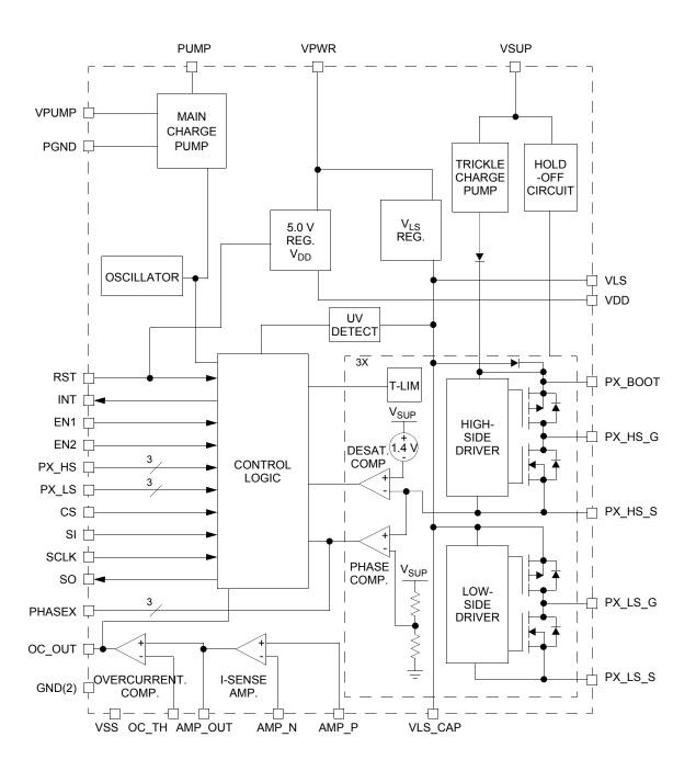
Figure 2. 34GD3000 simplified internal block diagram
