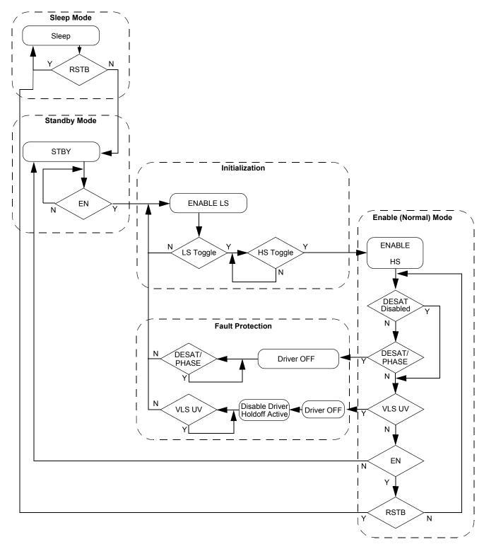
Figure 16. Device operational flow diagram
