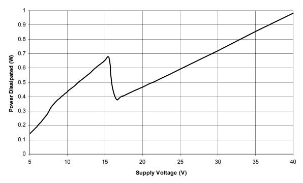
Figure 22. Power dissipation profile of application using charge pump
