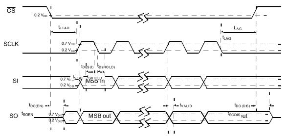
Figure 4. SPI interface timing
