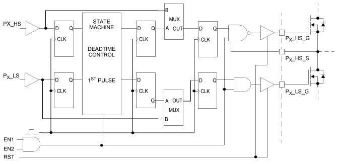
Figure 6. Deadtime control delays
