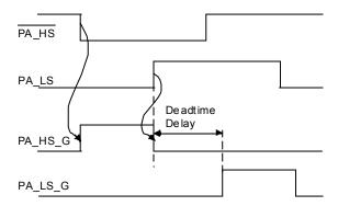
Figure 12. Edge sensitive logic inputs (Phase A)
