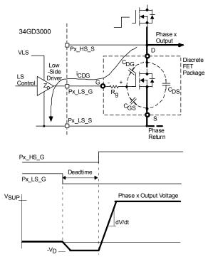
Figure 13. Positive dV/dt transient
