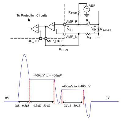
Figure 9. Current amplifier and input waveform (V $_{\rm IN}$  voltage across R $_{\rm SENSE}$ )
