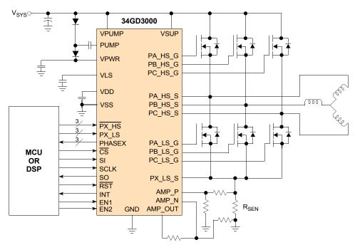
Figure 1. 34GD3000 simplified application diagram
