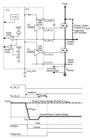
Figure 15. Short to supply detection
