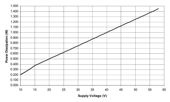
Figure 23. Power dissipation profile of application not using charge pump
