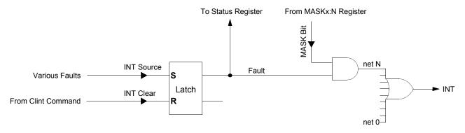
Figure 17. Interrupt handling
