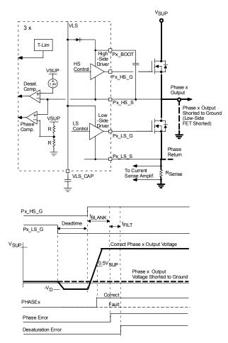
Figure 14. Short to ground detection
