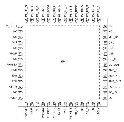
Figure 3. 34GD3000 pin connections
