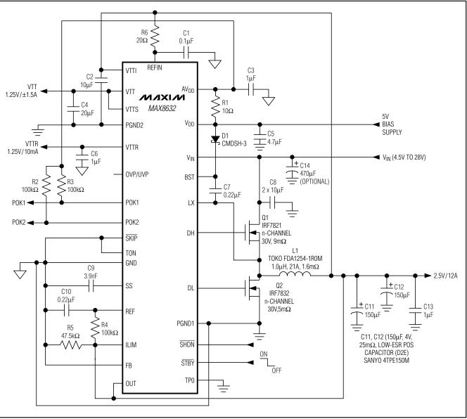
Figure 8. Typical Applications Circuit
