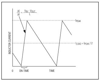
Figure 2. Pulse-Skipping/Discontinuous Crossover Point
