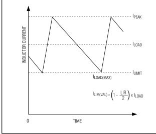
Figure 4. Valley Current-Limit Threshold
