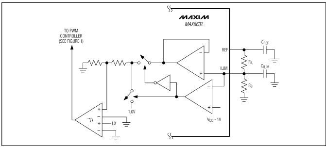
Figure 3. Adjustable Current-Limit Threshold
