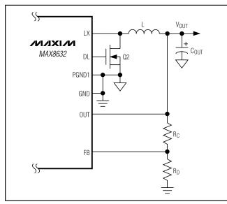
Figure 6. Setting VOUT with a Resistive Voltage-Divider
