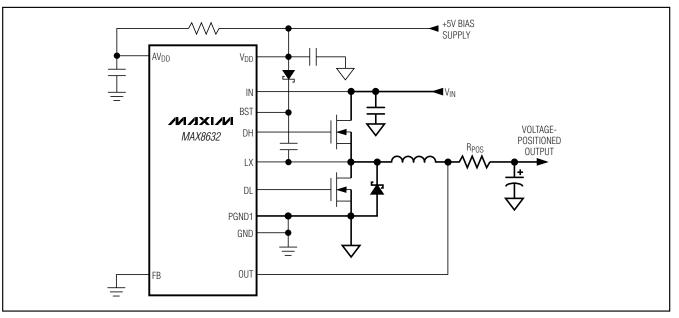
Figure 9. Voltage-Positioned Output
