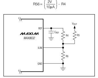
Figure 7. Foldback Current Limit
