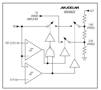
Figure 5. Dual-Mode Feedback Decoder
