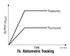
Figure 7. Two Different Modes of Output Voltage Tracking
