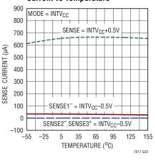
SENSE1,2+ and SENSE3- Input Current vs Temperature
