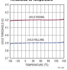
RUN Pin Thresholds vs Temperature
