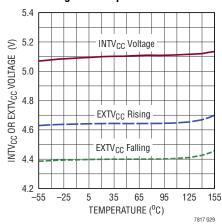
INTV<sub>CC</sub> Undervoltage Lockout Thresholds vs Temperature
