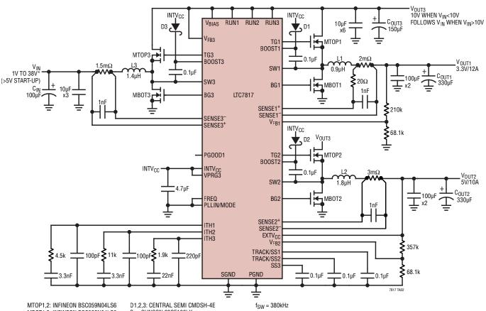
MBOT1,2: INFINEON BSC022N04LS6 MTOP3: INFINEON BSC022N04LS6 MBOT3: INFINEON BSC059N04LS6 L1: WURTH 744355090
