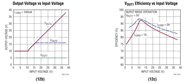
Figure 12. Wide Input Range 10V-16V Pass-Thru Cascaded Regulator and 5V Buck Regulator
