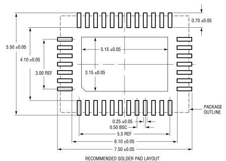
APPLY SOLDER MASK TO AREAS THAT ARE NOT SOLDERED
