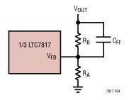
Figure 4. Setting Buck Output Voltage
