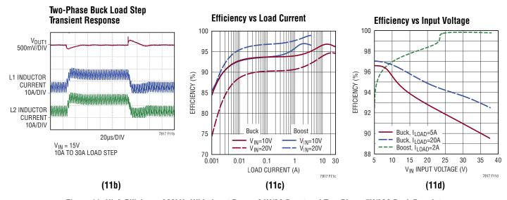
Figure 11. High Efficiency 380kHz Wide Input Range 24V/2A Boost and Two-Phase 5V/30A Buck Regulator
