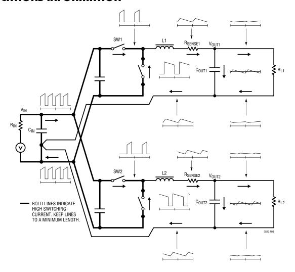
Figure 9. Branch Current Waveforms for Bucks
