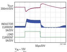
$V_{OUT} = 5V$ 300mA TO 6A LOAD STEP FIGURE 10 CIRCUIT
