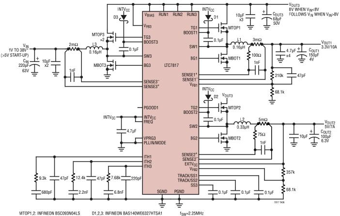
MTOP1,2: INFINEON BSC093N04LS MBOT1,2: INFINEON BSC093N04LS MTOP3 (x2): INFINEON BSC027N04LS MBOT3: INFINEON BSC059N04LS L1,3: COILCRAFT XAL5030-161ME L2: COILCRAFT XAL5030-331ME
