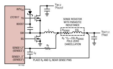
2a. Using a Resistor to Sense Current
