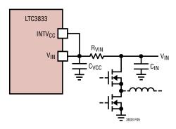
Figure 5. Setup for  $V_{IN} \le 5V$
