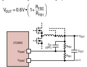
Figure 1. Setting Output Voltage
