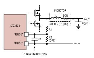
Figure 4. DCR Current Sensing
