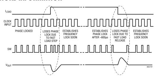
Figure 7. Phase and Frequency Locking Behavior During Transient Load Conditions
