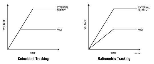
Figure 6a. Two Different Modes of Output Tracking
