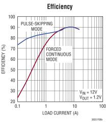
Figure 9. 1.2V, 15A, 350kHz Step-Down Converter
