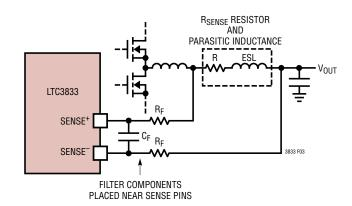
Figure 3. R<sub>SENSE</sub> Current Sensing
