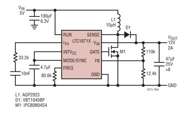
High Efficiency 5V Input, 12V Output Boost Converter (Bootstrapped)
