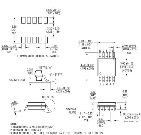
**MS Package 10-Lead Plastic MSOP** (Reference LTC DWG # 05-08-1661 Rev F)
