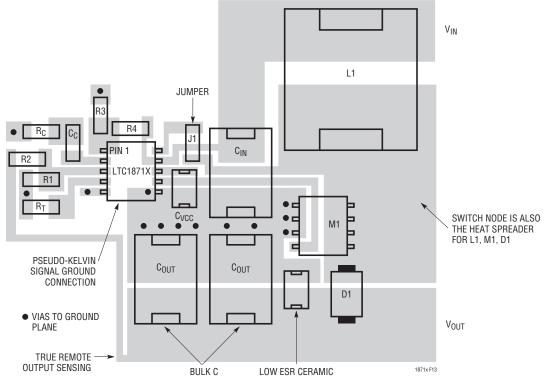
Figure 13. LTC1871X Boost Converter Suggested Layout
