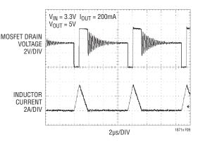
Figure 9. Discontinuous Mode Waveforms
