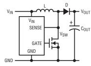
2a. SENSE Pin Connection for Maximum Efficiency (V<sub>SW</sub> < 36V)
