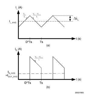
FIGURE 4. (a) Inductor current. (b) Diode current.
