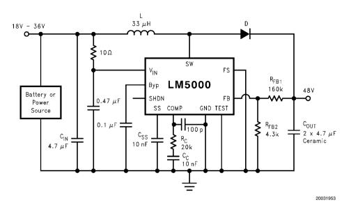
FIGURE 1. 300 kHz operation, 48V output
