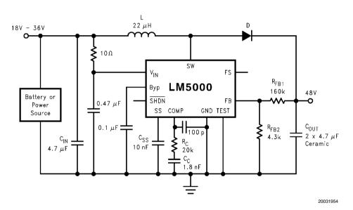
FIGURE 2. 700 kHz operation, 48V output
