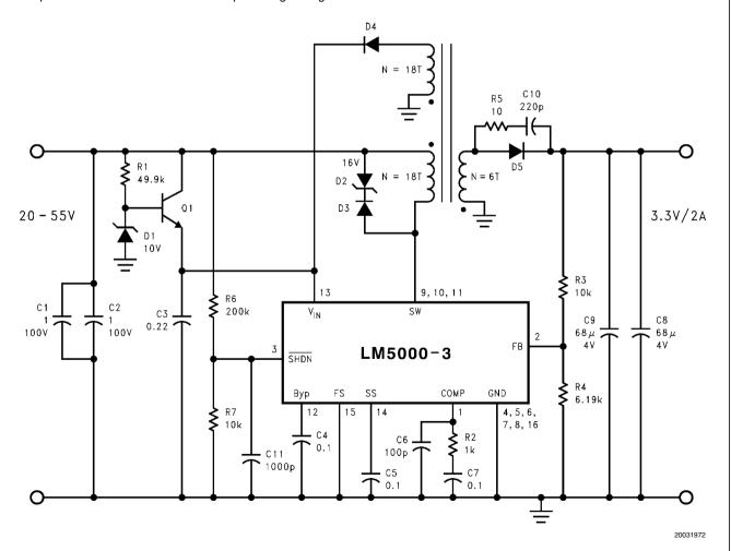
FIGURE 5. LM5000 Flyback Converter
