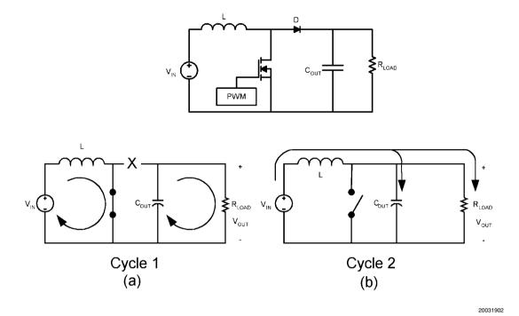
FIGURE 3. Simplified Boost Converter Diagram
