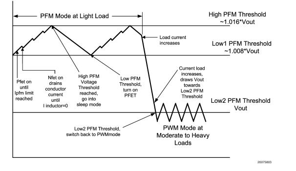
FIGURE 5. Operation in PFM Mode and Transition to PWM Mode
