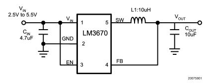
FIGURE 1. Fixed Output Voltage - Typical Application Circuit
