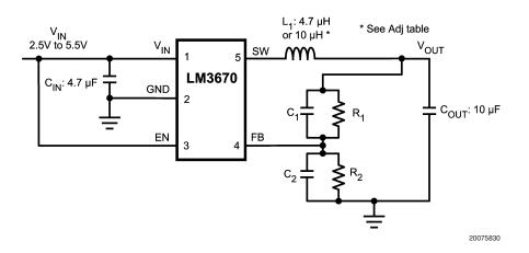
FIGURE 2. Adjustable Output Voltage - Typical Application Circuit
