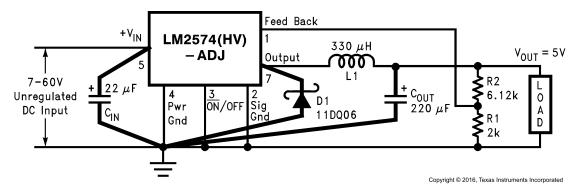
Figure 34. LM2574 Adjustable Output Voltage Layout
