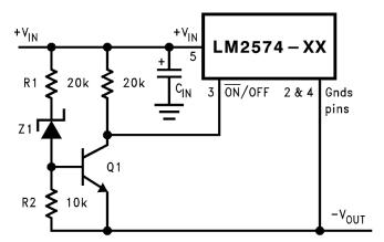
**Note:** Complete circuit not shown (see Figure 20). **Note:** Pin numbers are for 8-pin PDIP package.
