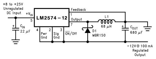
Note: Pin numbers are for the 8-pin PDIP package.
