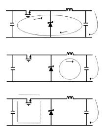
Figure 33. Buck Converter Current Flow
