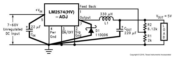
Figure 27. Adjustable Output Voltage Version
