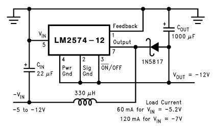
Note: Pin numbers are for 8-pin PDIP package.
