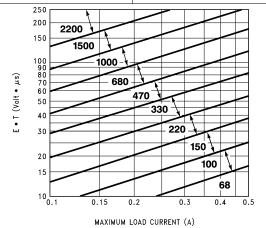
Figure 32. Adjustable LM2574HV Inductor Selection Guide
