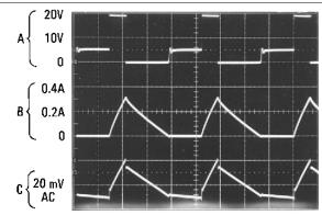
Output pin voltage, 10 V/div, Inductor current, 0.2 A/div, Output ripple voltage,
