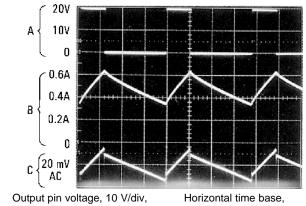
Inductor current, 0.2 A/div, Output ripple voltage,
