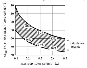
Figure 19. Inductor Ripple Current (Δi<sub>IND</sub>) Range
