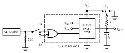
$\ensuremath{C_L}$  includes load and test jig capacitance.
