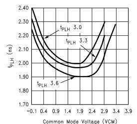
Figure 10. Variation in Low to High Propagation Delay versus VCM
