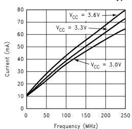
Figure 6. ICC vs Frequency, four channels switching
