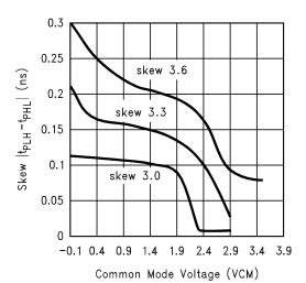
Figure 8. Typical Pulse Skew variation versus commonmode voltage
