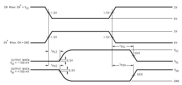
Figure 4. Receiver TRI-STATE Delay Waveforms
