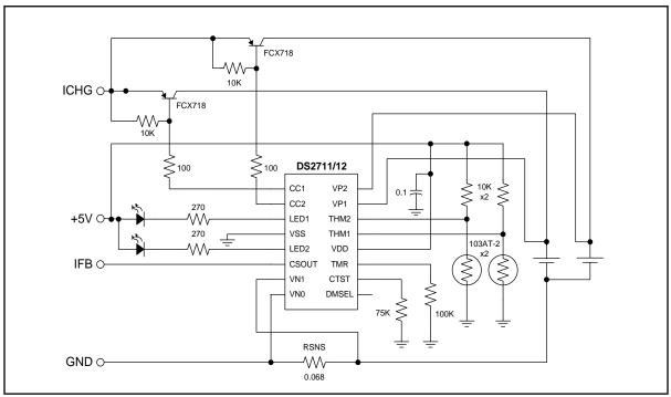
The series or parallel charge configuration is programmed by strapping LED2 in the low, high, or high-Z state during power-up. In this example and the following one, the parallel charge mode is selected by pulling LED2 pin high during power-up. This is accomplished in this example by the LED and  $270\Omega$  resistor. In applications where only one LED is used, a  $100k\Omega$  pullup resistor is recommended. See Table 2 for additional configuration programming information.
