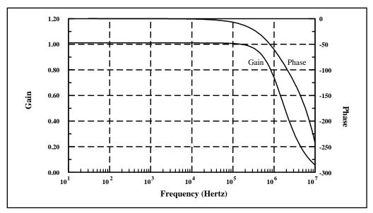
The open-loop amplifier response shown in Figure 6 was measured with  $I_{CSOUT} = -1mA$ . An error signal between the current-sense signal (across a sense resistor) and the 0.125V internal reference is produced so the voltage across the sense resistor is maintained at  $V_{IREF}$  in a closed-loop circuit.
